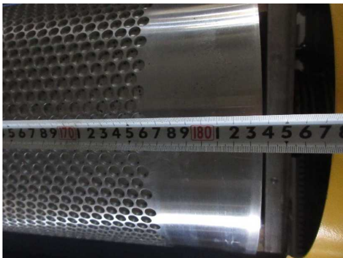
264 ↑ Cooling roller size check-Passed
