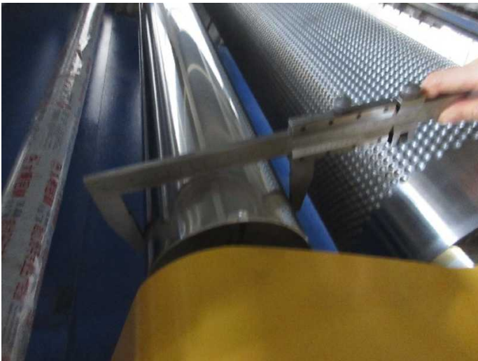
271 ↑ Cooling roller size check-Passed
