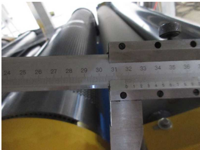
260 ↑ Cooling roller size check-Passed
