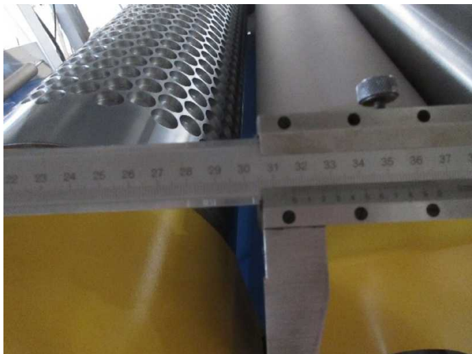
262 ↑ Cooling roller size check-Passed
