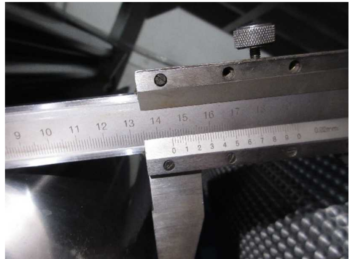
272 ↑ Cooling roller size check-Passed
