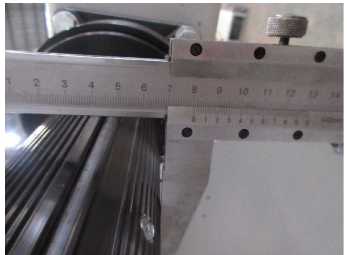
274 ↑ Air shaft size check-Pending
