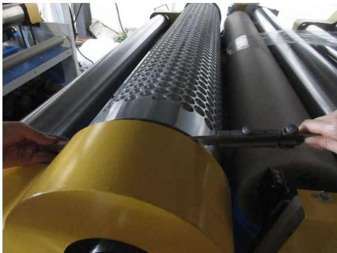
261 ↑ Cooling roller size check-Passed
